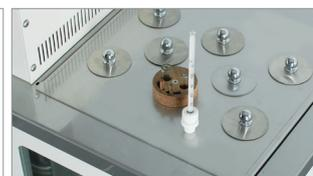
Easy holding of U-shaped viscometer glass tubes (optional)
